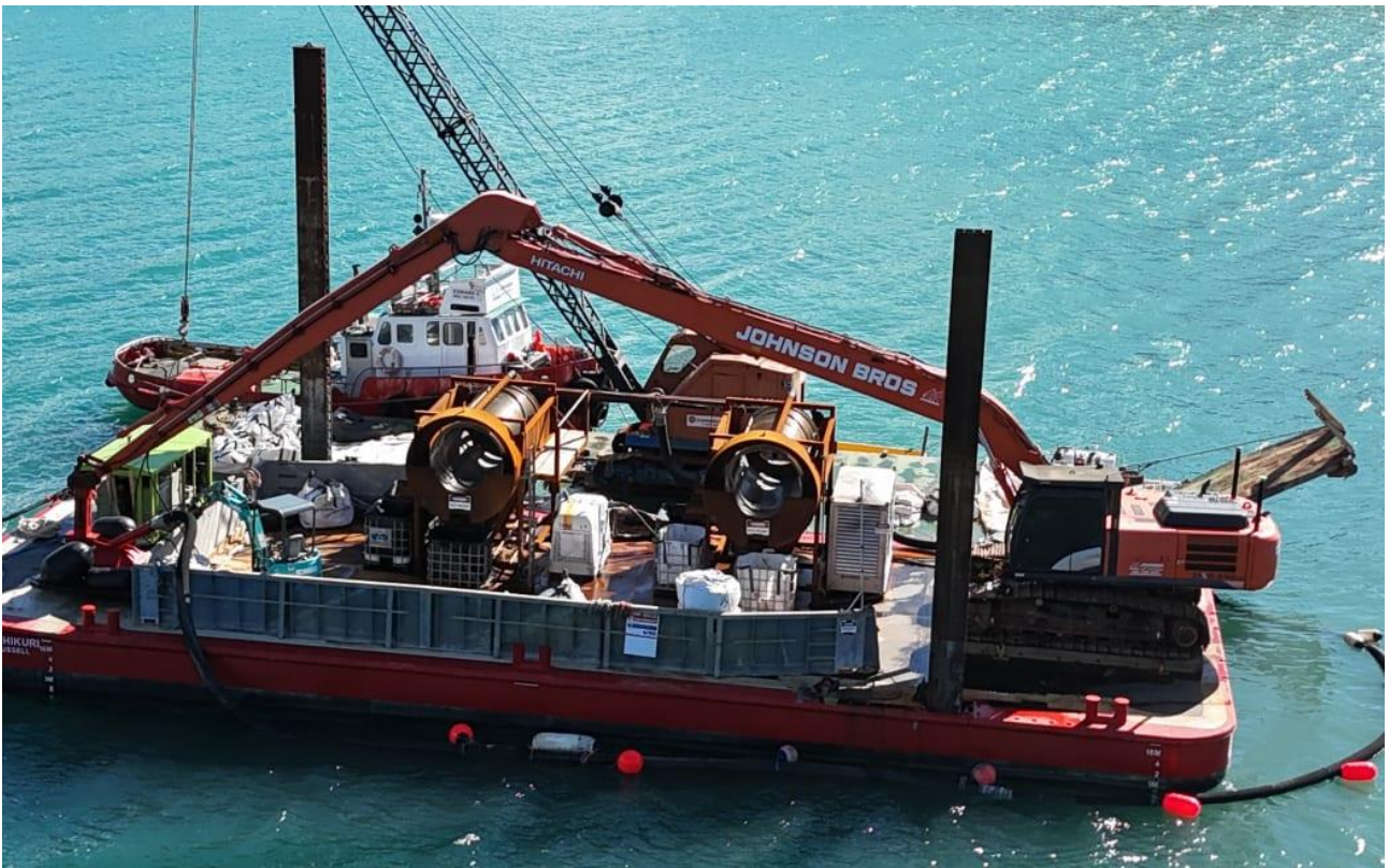
Figure 1: Mahikuri barge set up for unique project (Caulerpa suction dredging trials)
